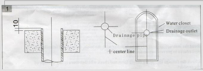
1.Mark the + centre line according to the drainage outlet on the floor and that of the toilet. NOTE: The drainage pipe should be higher about 10mm from floor for better sealing.
