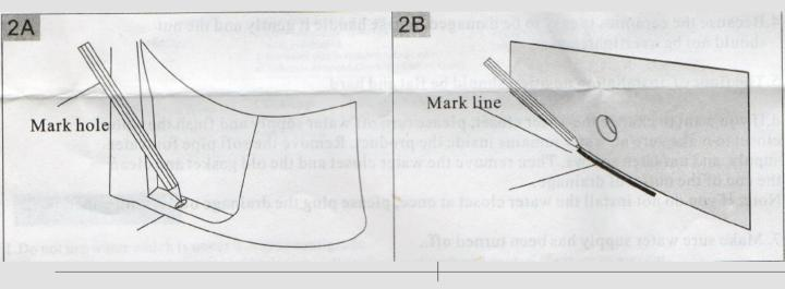
2.Put the toilet into the installation position. Make sure the + center lines of floor and toilet are aligned properly. Then mark the installation holes with pencil.
