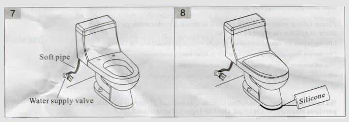
7. Install the water supply valve. Connect the filter and water supply soft pipe of cistern. Check the connection carefully to make sure there is no leakage. 8. Install toilet seats according to the installation instructions, then dab a layer of silicone between the product and floor.
