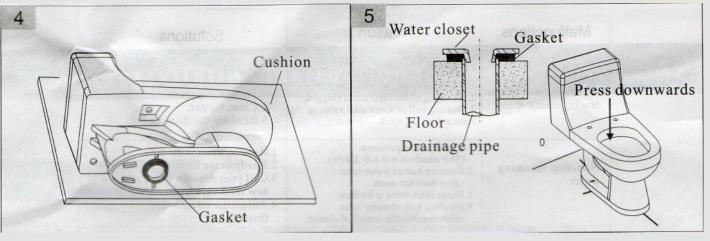
4. Put the product onto the cushion flatly, then place the wax ring gasket onto the drainage outlet tightly.
